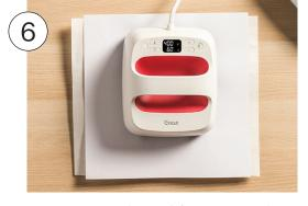
Press at 400°F (205°C) for 60 seconds. Tip: If you are using a larger Cricut EasyPress, you can transfer Infusible Ink designs to multiple coasters at the same time.
