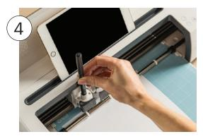
Insert Infusible Ink Pen or Marker into Clamp A, then press flashing **Go** button. Note: If you have assigned multiple pen colors to your design, Design Space will prompt you to load specific colors at specific times.
